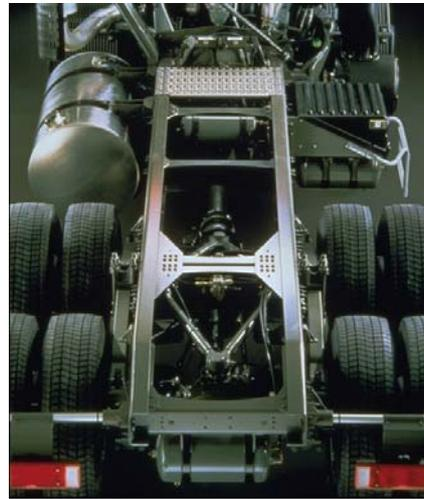
Fig 9 Truck frame in Domex 690 XP
