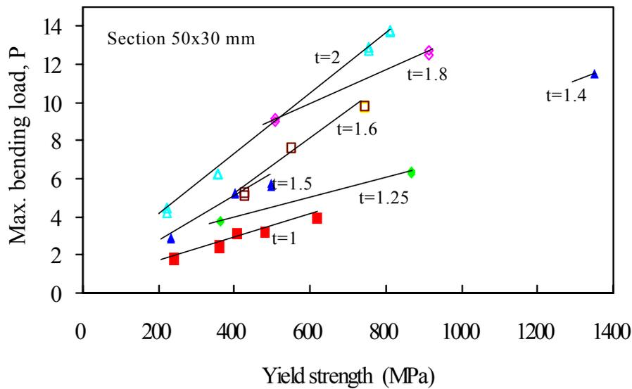
Fig 7 Maximum load  $P_{max}$  vs. yield strength for bending tests
