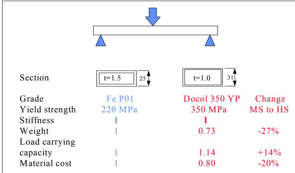
Fig 3 Reduced weight and cost with unchanged stiffness
