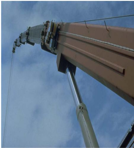
Fig 8 Crane boom in Weldox 700 and Weldox 900
