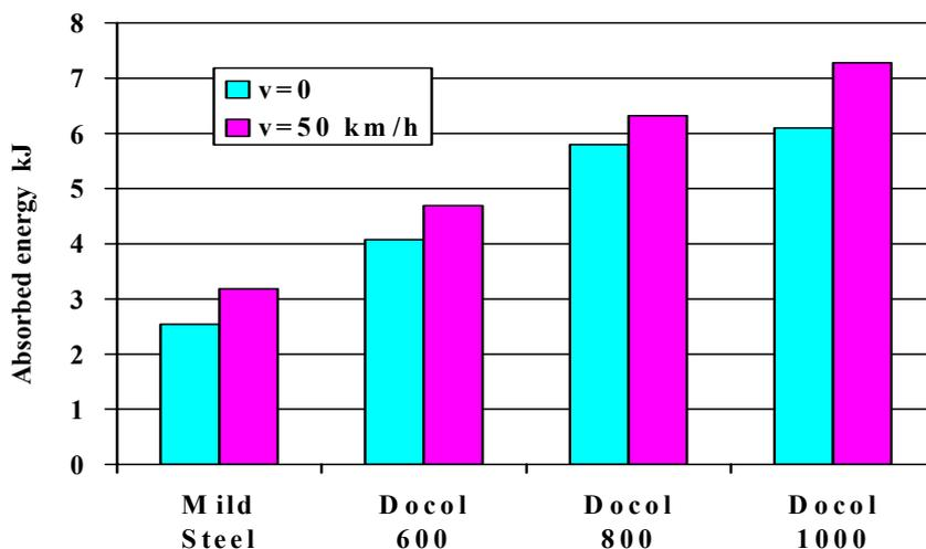
Fig 6 Absorbed energy in axial crush tests on rectangular hollow sections in DP steels
