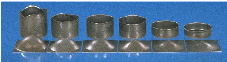
Fig 1 Examples from tests in deep drawing and stretch forming of steels DC O4 (mild steel), Docol 600 DP, Docol 800 DP, Docol 1000 DP, Docol 1200 DP and Docol 1400 DP
