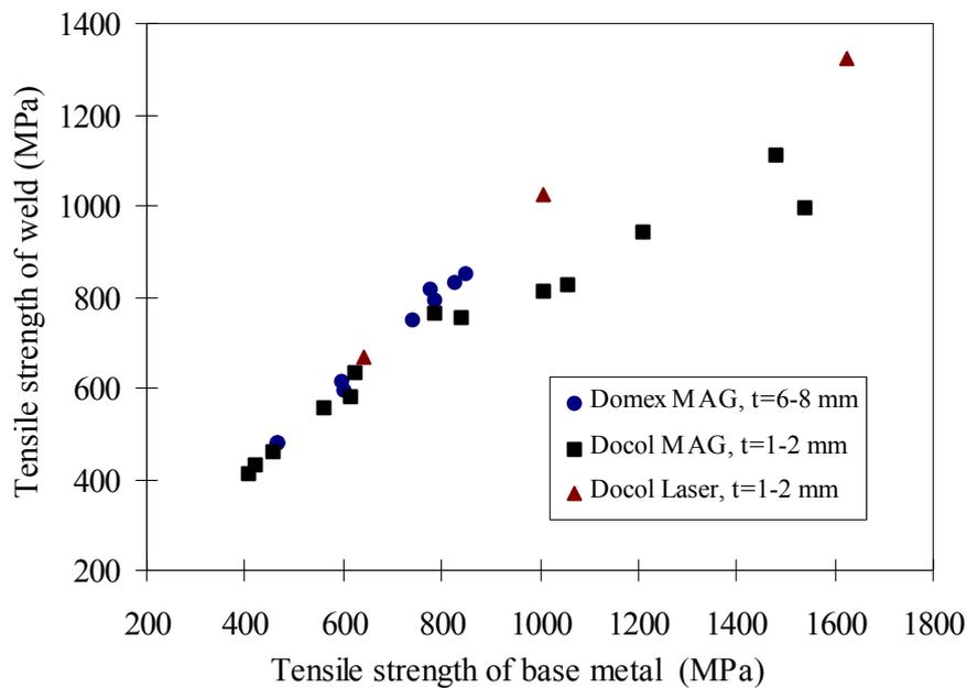
Fig 2 Tensile strength of MAG and Laser welds as a function of base metal tensile strength.
