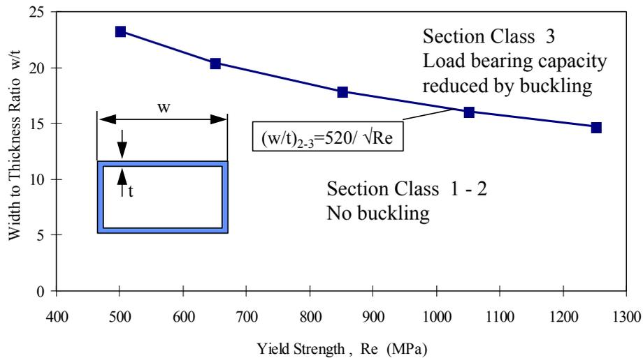
Fig 4 Limiting width to thickness ratio (w/t) for buckling
