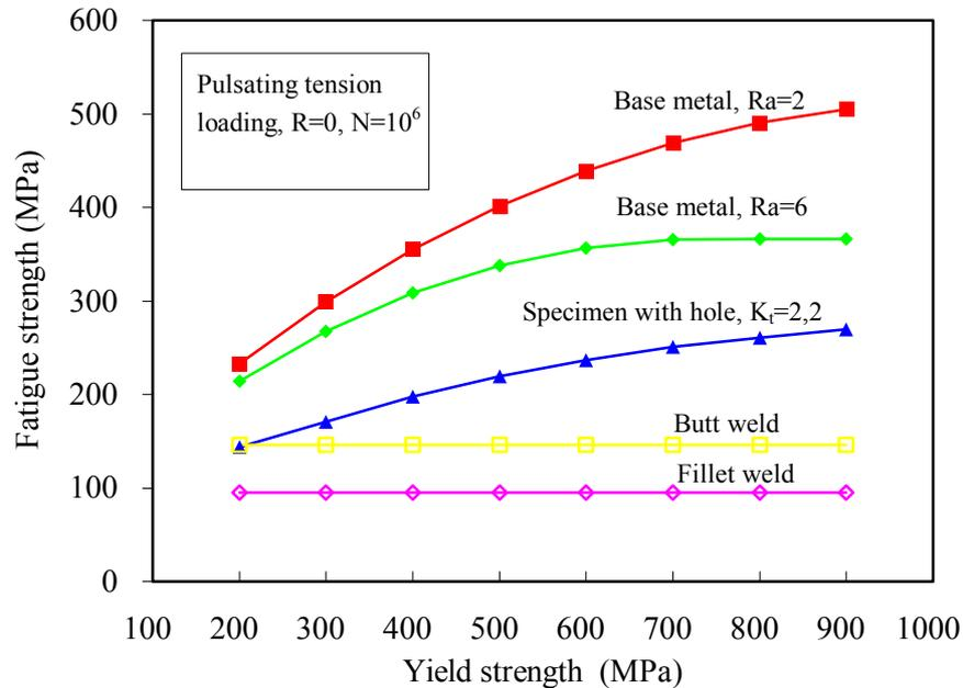
Fig 5 Fatigue strength as a function of yield strength
