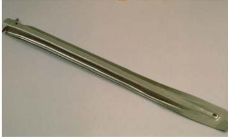
Fig 10 Door intrusion beam in Domex 690 XP
